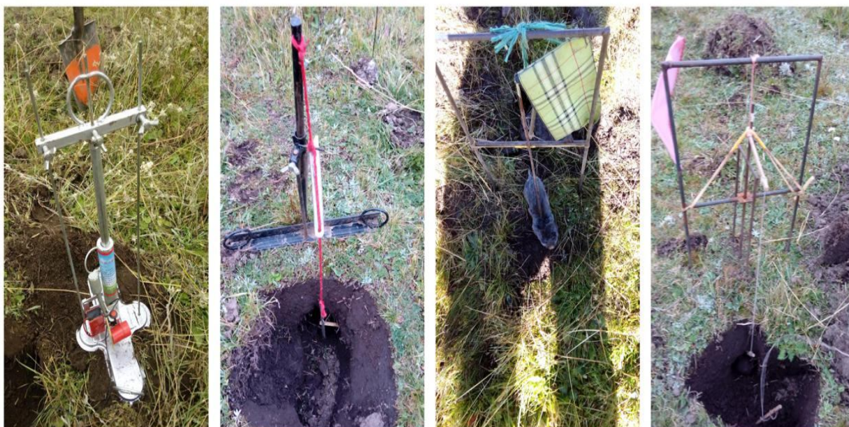
Fig. 1. Different arrow traps. From left to right: the intelligent (infrared) type, the T-type, the one-arrow type, the three-arrow type.
